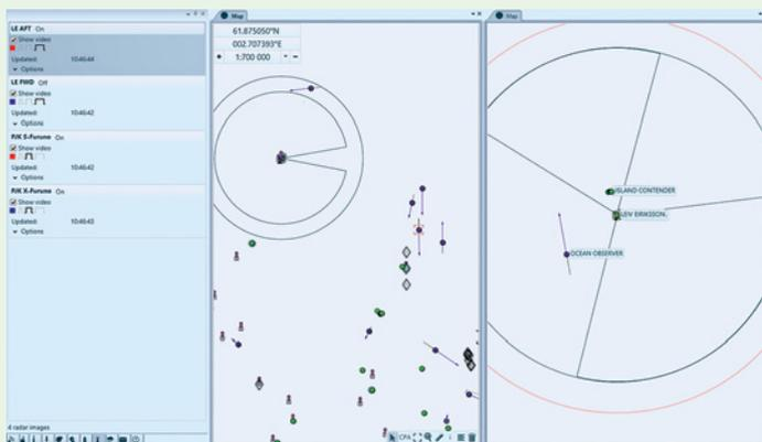
The iSurv Information Surveillance Display is an intuitive operator display, all system functions and components including 3rd party modules can be accessed and controlled from iSurv. The operator display presents tracked targets from radars and AIS on S-57 electronic charts. Ten security levels provide data protection and each user can customize their work space.
